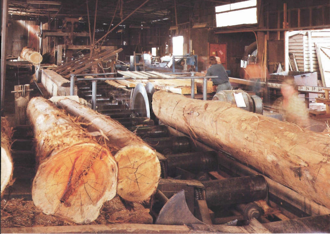
Twin circular saws about to make the first cuts through a messmate stringybark log at a small hardwood mill.
