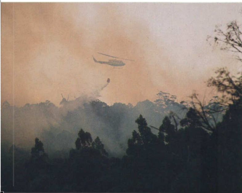
A Bell 212 helicopter carrying a 1,900 litre bucket drops water on a fire in a mountain forest.
